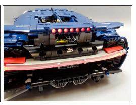
• The pre-lit spoiler should still move up and down as freely as it did before you installed the LEDs. Check to make sure you can still open and close the spoiler, and that it stays up when open.
