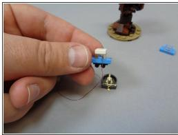
Take the pre-lit car and battery holder assembly out of its bag, and as shown in the second photo, remove the white top and black wheels from the car in your LEGO® set and transfer them to the pre-lit car as shown in the third photo.
