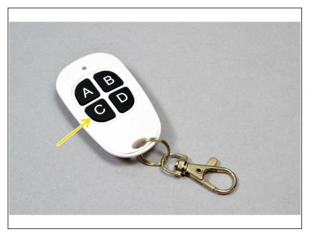
The remote control supports two special configuration modes, each of which is accessed by holding down the given button while power is OFF to both the Falcon lights and sounds, then continuing to hold the button for 3 seconds after power has been turned on.
