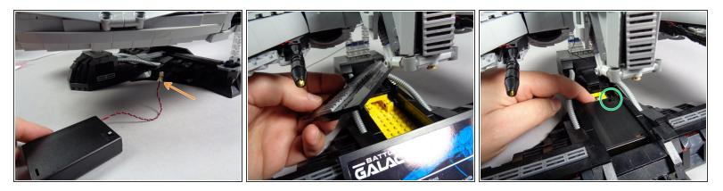
• As shown by the orange arrow in the first photo, connect the plug from the battery pack wire to the other end of the BRANCH13 adapter.
