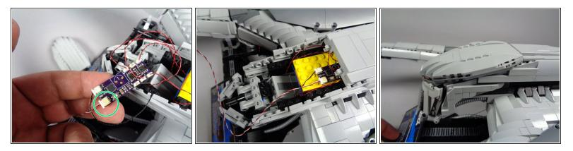
• As shown by the green circle in the first photo for this step, connect the 3-wire plug that connects to the eye assembly to the other large plug on the effect controller.
