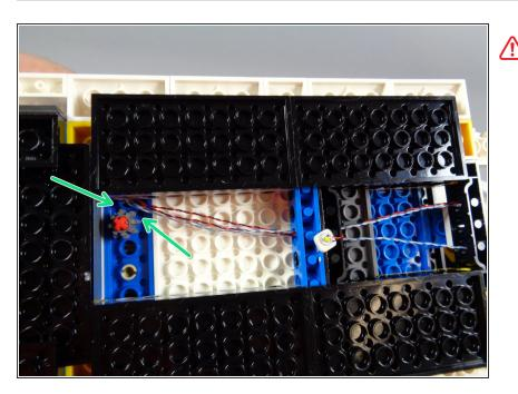
As shown by the green arrows in the photo for this step, make sure the wires are not stuck in the gear. It is critical that the roof radar be able to rotate freely without catching any of the wires.
