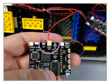
As shown by the purple circle in the photo for this step, connect the red control wire from the roof lights to the ROOF LIGHTS plug on the main controller.
