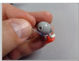
As shown in the photos for this step, finish re-assembling the hood spot light, taking care to make sure the light wire passes between the clip prongs and that the wire is not pinched when the light is re-attached to its bracket.
