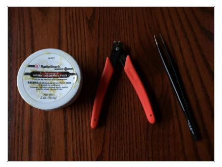
In addition to a good soldering iron, we recommend also having some soldering flux on hand, along with a good pair of angle-cut clippers and a good pair of tweezers. We use the <u>Xuron XUR410T sprue cutter</u> and the <u>Wiha 44518 tweezers</u>.
