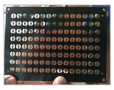
This is a full panel of Pico LEDs (120 in total). You may have purchased less than a full panel, but this photo shows how each Pico LED is attached to the panel with two "fingers"-- one on the top of each Pico LED and one on the bottom.
